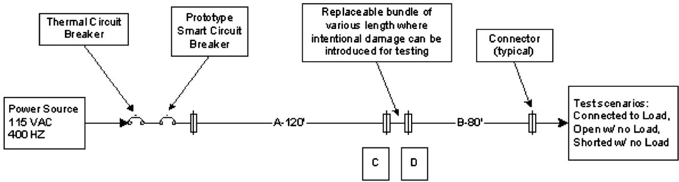
Fig. 3. Boeing wiring test bench.
