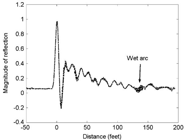
Fig. 7. STDR traces showing the instantaneous near short circuits caused when saline solution is dripped on a wire with damaged insulation, making a partial path for conduction. Several time samples are superimposed to show the location of the wet arc.
